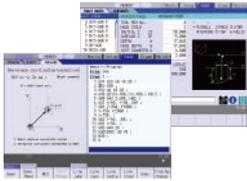
Create NC programs while referring to drawings. Possible to use G code and dimension input (NAVI MILL/NAVI LATHE).
