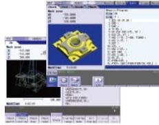
Visually check whether or not the NC program created operates correctly.
