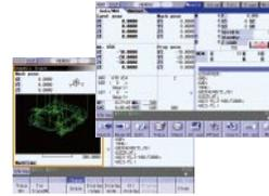
Possible to learn a series of operations via NC programs created and execute graphic tracing during operation.
